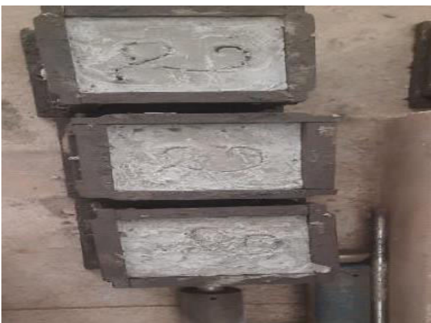
Figure-1. Cube casting.
