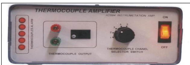
Figure-1. Thermocouple amplifier instrument.
