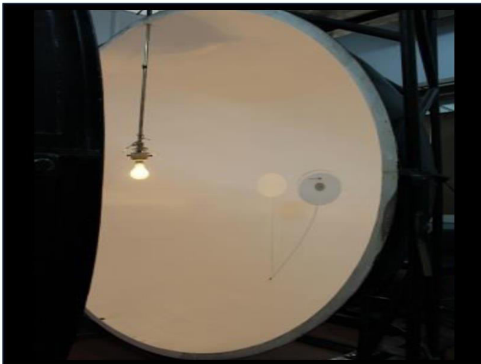
Figure-1. NIS 2.5 m integrating sphere photometer set up.
