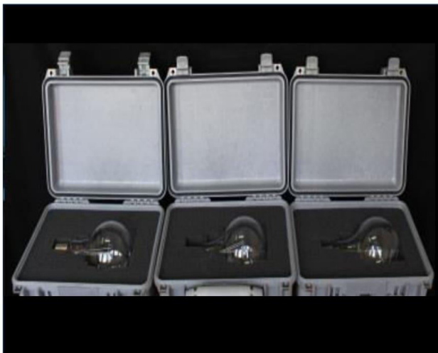
Figure-2. NIS luminous flux secondary standards lamps.
