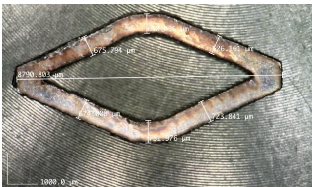
Figure-2. Measurement of the width (dimension/Dim.) of the diamond feature profile.
