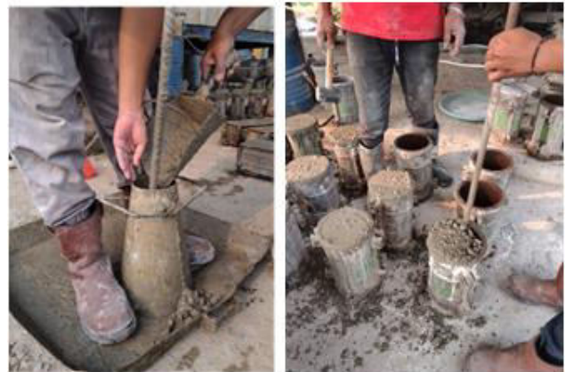
Figure-2. (a) Slump test (b) Specimens casting.
