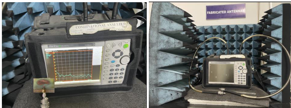
Figure-12. Measurement of VSWR and Fabrication setup of the proposed antenna.
