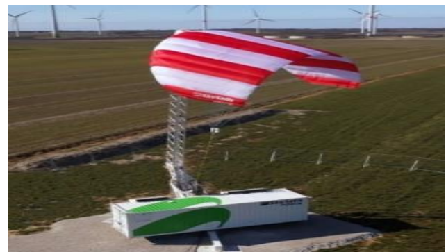
Figure-3. Skysails power kites harvest wind energy at altitudes of up to 400 meters.
