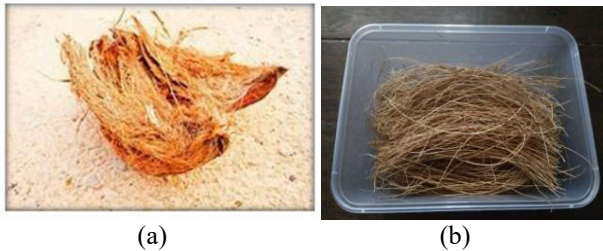
Figure-1. (a) Old coconut fibre and (b) Coconut fibre with 140mm cutting.
