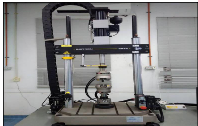
Figure-4. Universal Tensile Testing Machine with a load capacity of 25 kN.
