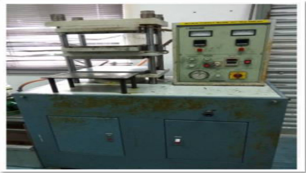
Figure-3. Motorised hydraulic molding test press machine for composites fabrication.
