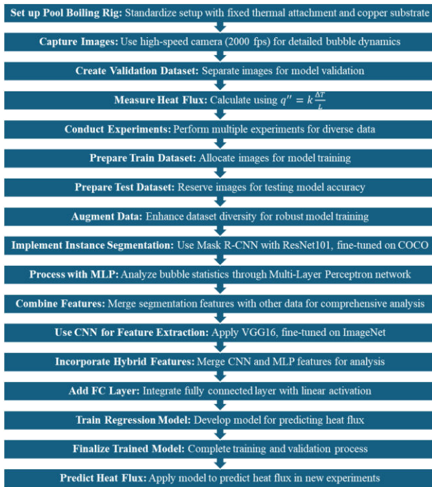
Figure-3. Comprehensive workflow of pool boiling experiment: from setup to heat flux prediction.
