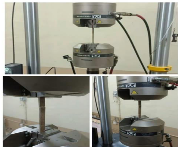
Figure-9. Tensile test of the specimens using UTM.
