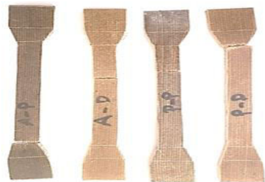
Figure-10. Specimens after tensile test.
