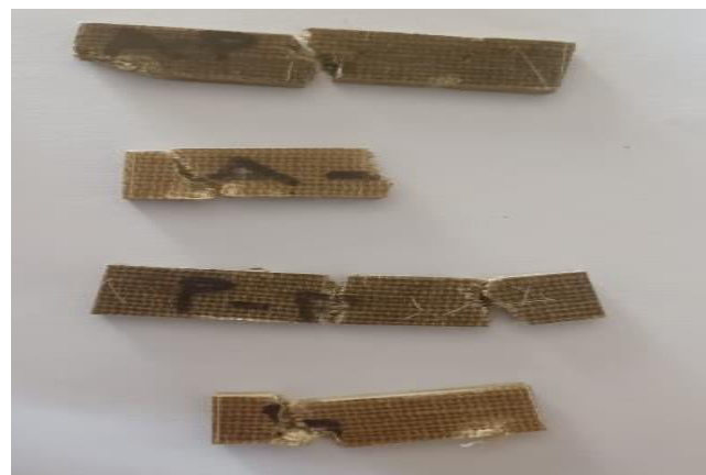
Figure-17. Specimens after impact test.
