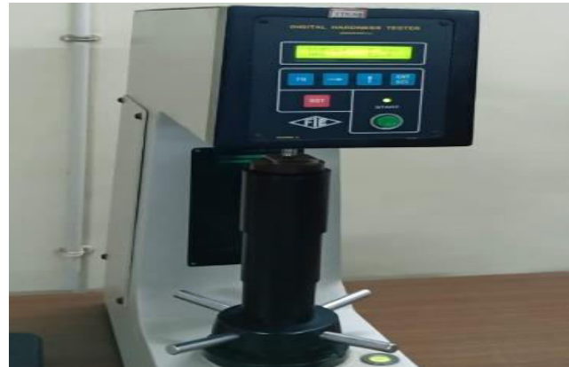
Figure-14. Hardness test using rockwell machine.
