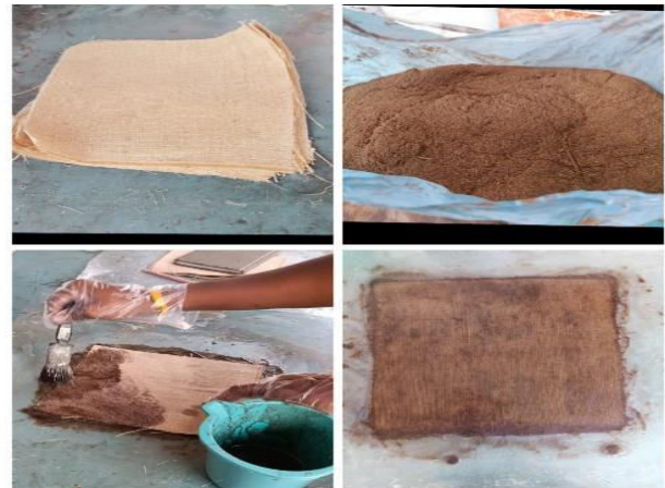
Figure-1. Preparation of laminates by using Araldite LY556, Polyester, and Areca trunk husk.
