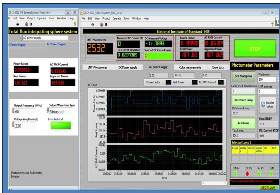
Figure-2. LABVIEW software control system for total flux developed NIS-integrating sphere photometer system [8].
