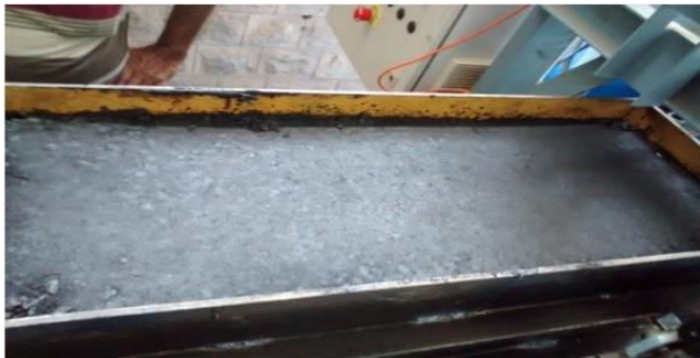
Figure-2. Specimen before rutting.
