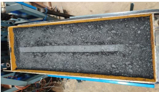
Figure-3. Specimen after rutting.
