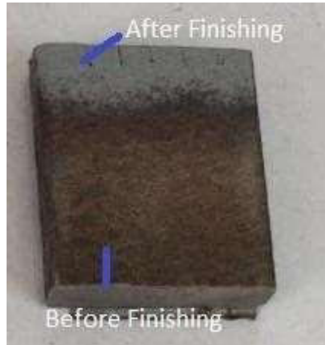
Figure-3. Sample before and after finishing at 6 bar pressure.
