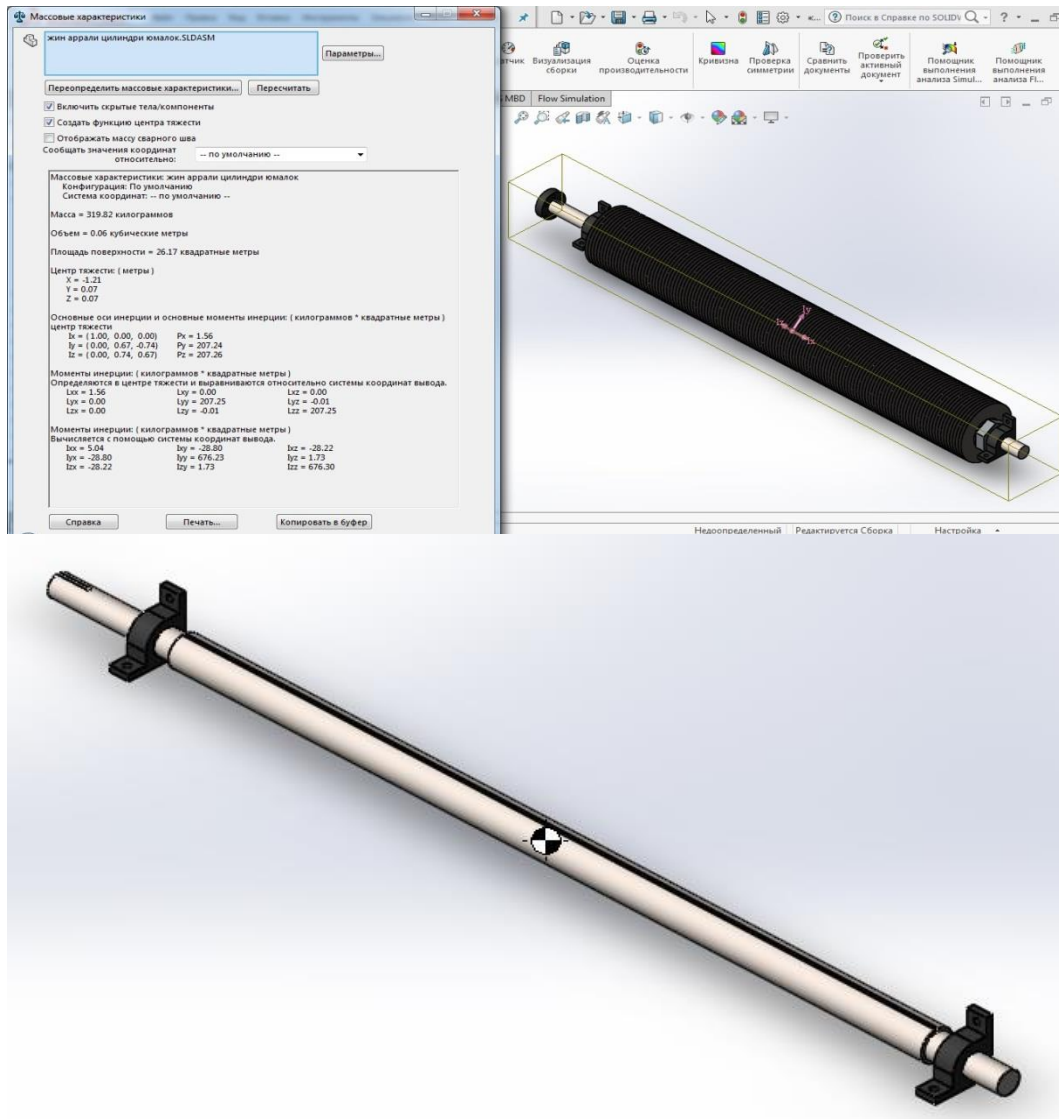
Figure-10. Calculation of balancing the shaft of a circular saw cylinder.
