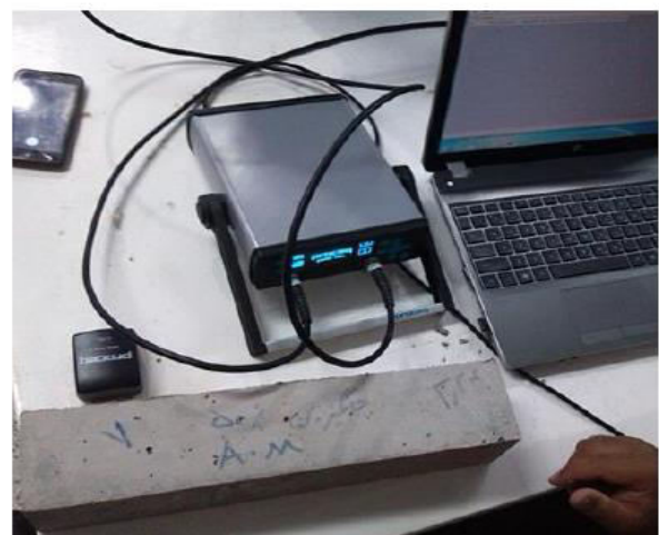
Figure-4. Sonic inspection device.
