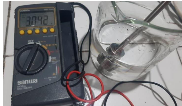
Figure-5. Level sensor testing.
