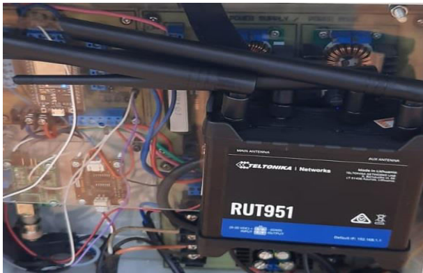
Figure-7. Data communication system using a modem.
