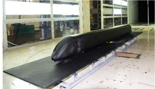
Figure-13. HST model experiment setup in the wind tunnel.
