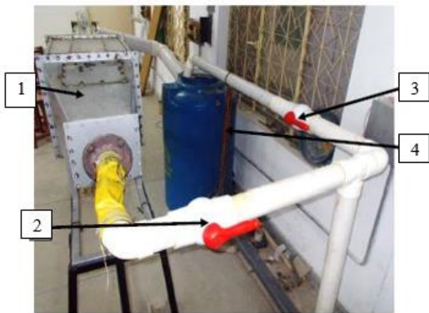
Figure-2. Mechanism for flow control (1) Test Rig (2) Valve 1 (3) Valve 2 (4) Water Reservoir.
