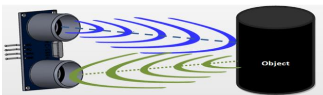
Figure-3. Distance calculation using ultrasonic sensor.
