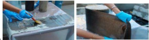
Figure-3. a) fabric saturated with epoxy3 b)wrapping around the surface.
