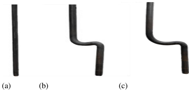
Figure-1. Test teeth: a) a straight tooth; b) a tooth, with a working part curved by a radius of 30 mm; c) a tooth with a working part of a curved radius of 50 mm.
