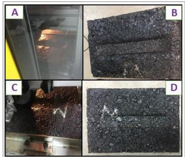
Figure-7. Final rut depth for (A), (B) slabs with conventional mixture (C), (D) slabs with HMAC mixture.
