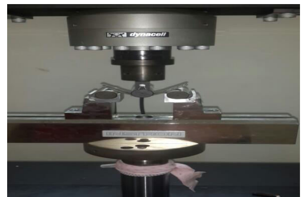
Figure-4. Flexural test.
