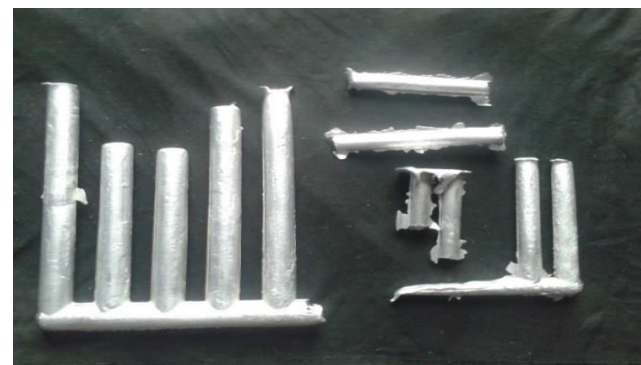
Figure-2. Cast hexenary aluminium alloy.
