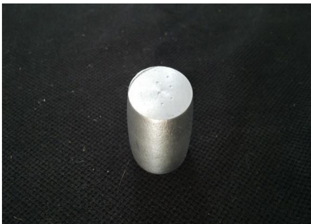
Figure-6. Compression test specimen after deformation.
