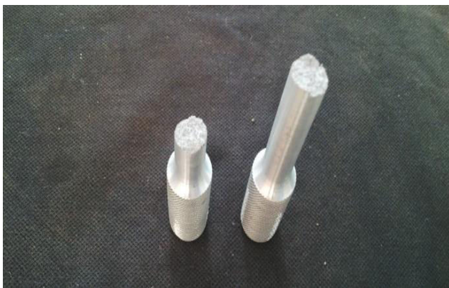
Figure-5. Tensile test specimen after fracture.
