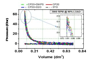
Figure-9. P-V diagram with load.
