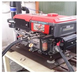
Figure-2. Yanmar diesel engine TF12ML. Table-3. Test engine specification.
