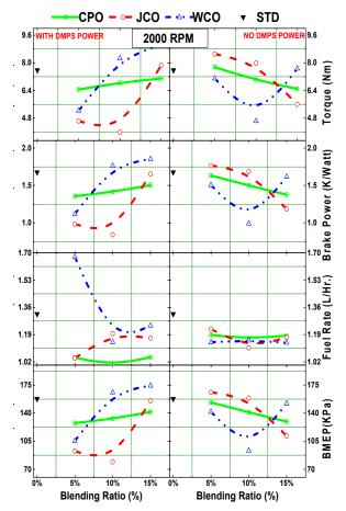
Figure-5. Performance with blending ratio at load 90% in high speed.
