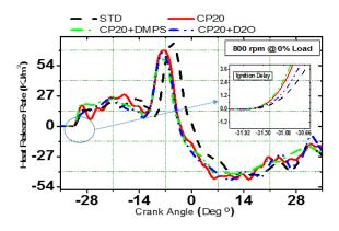
Figure-10. Heat release rate without load.
