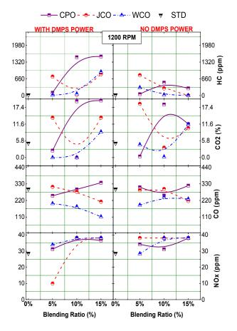
Figure-6. Emission with blending ration at load 50% in low speed.
