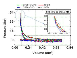
Figure-8. P-V diagram without load.
