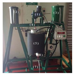
Figure-1. Laboratory scale blending machine.
