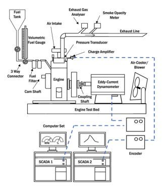
Figure-3. Schematic of experimental setup.
