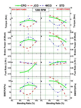
Figure-4. Performance with blending ratio at load 50% in low speed setup.
