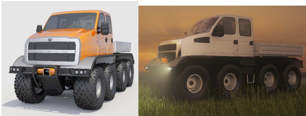
Figure-2. 3D model of the RUSAK-3993 terrain vehicle (8x8).
