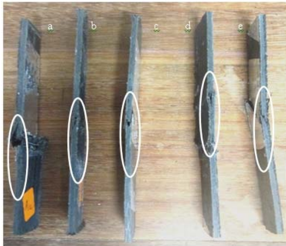
Figure-7. Typical compressive failure of laminates (a) brooming (b) kinking (c) inplane-shear (d) delamination (e) transverse shear.
