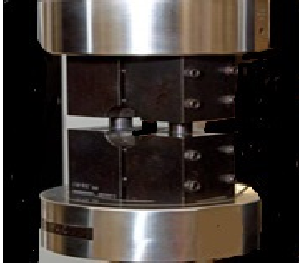
Figure-4. CLC fixture for compression test.
