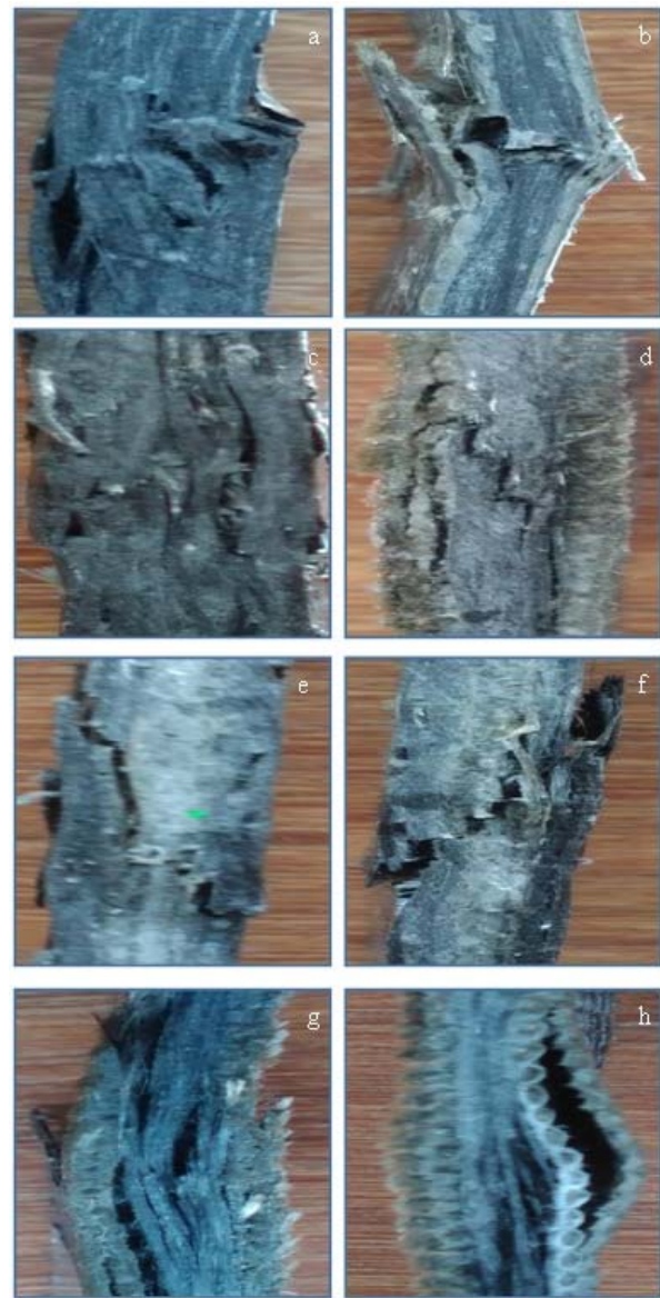
Figure-8. Compression failure modes of tested specimens.
