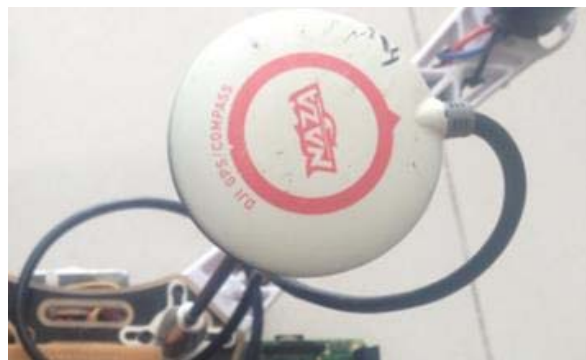
Figure-6. Naza GPS module mounted on the quadcopter.
