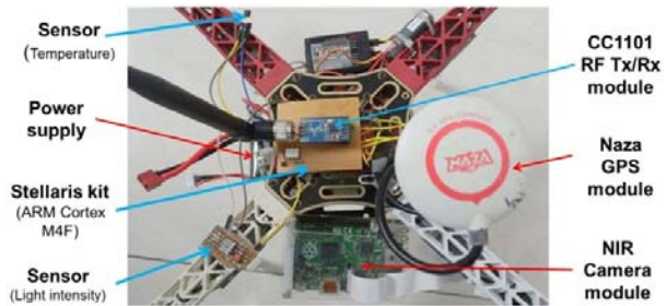
Figure-11. Positions of on-board modules installed on the quadcopter.
