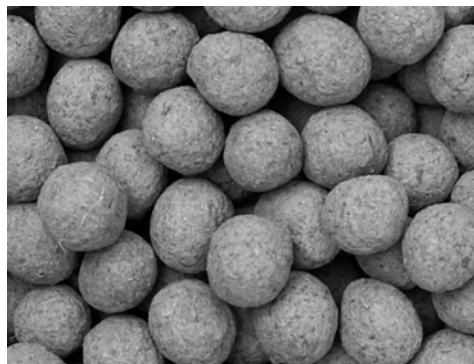
Figure-2. Spherical organometallic granules on the base of flax shive.
